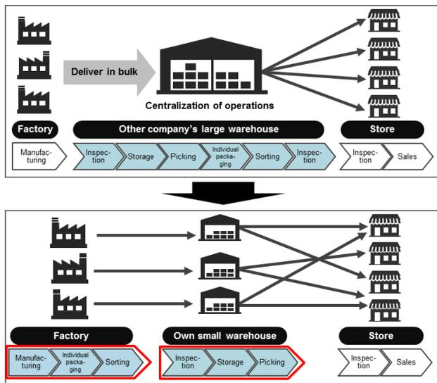
Figure 2 Consolidation/simplification of processes
